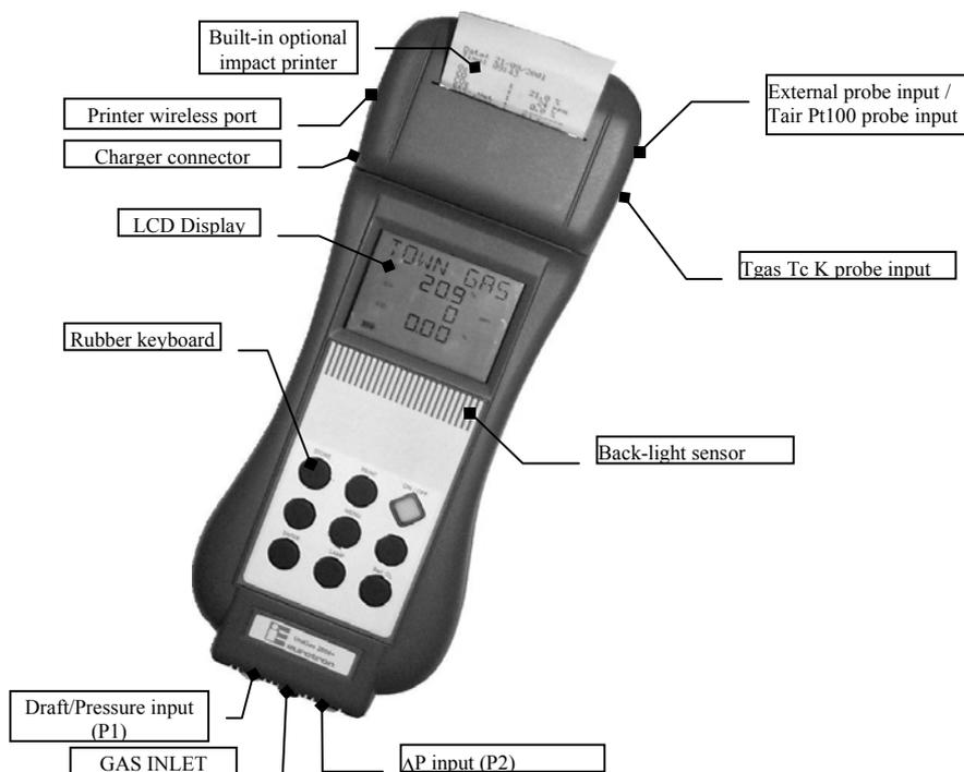
At the bottom of the instrument, you can see all sampling probe connectors: gas inlet, and differential pressure / draft inputs.
