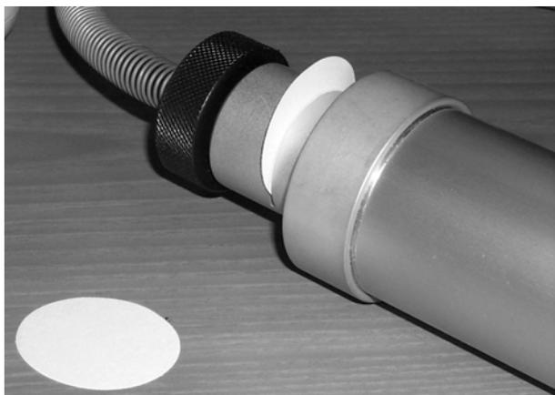
The gas sample should be drawn to the center of the combustion gas flux. The correct gas volume is sampled with 10 uniform shoots by the pump. We suggest using a retaining cone during gas sampling. Compare the darkening of the filter with the smoke index comparing table. The smoke index found should not exceed the ones defined by the current normative.
