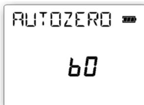
This page displays the seconds to end the autozero procedure.
