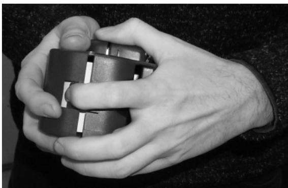
Extract the exhausted paper roll. You can use standard paper roll but you have to check before for its dimensions (max. 57mm  $\pm$ 1mm large).
